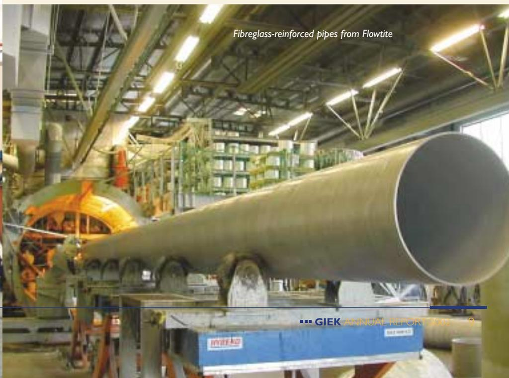
Fibreglass-reinforced pipes from Flowtite
